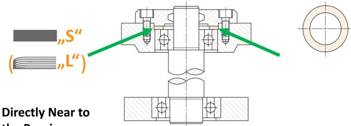
Directly Near to the Bearing: Can Bring Wear and Friction Problems Over Life Time
